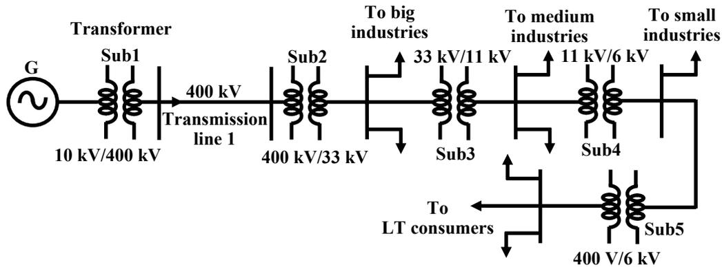
**Figure 2.9: Single line representation of power system.**
